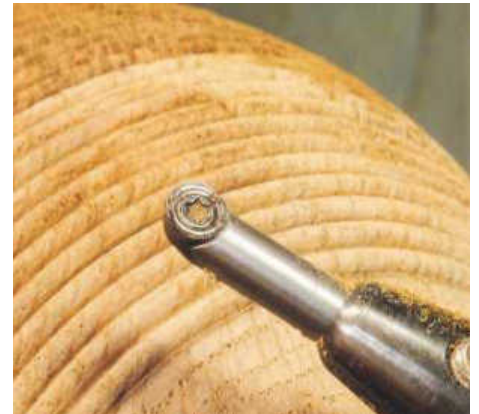
STEP 13. The Simon Hope hollowing tool is the best tool that I have found for doing this type of work. The small diameter cutter combined with the thick shaft makes the tool an absolute dream to use
